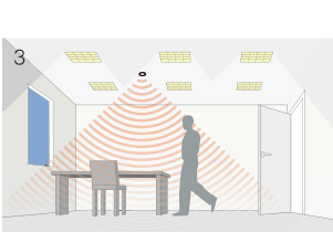
3. Enter the room or make some movement and check that the load switches on.
