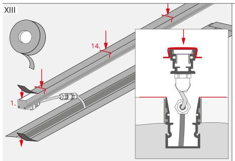
Secure the surface of the fixture and the edges of the mounting track with protective tape.
