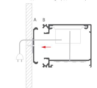
**9.** Secure the extrusion (B) against falling off by inserting the 4 mm plastic rods (F) into the guides and tightening them with M5 pressure screws (J) using the Allen wrench. Sink the pressure screws deep enough so there is room for end caps.
