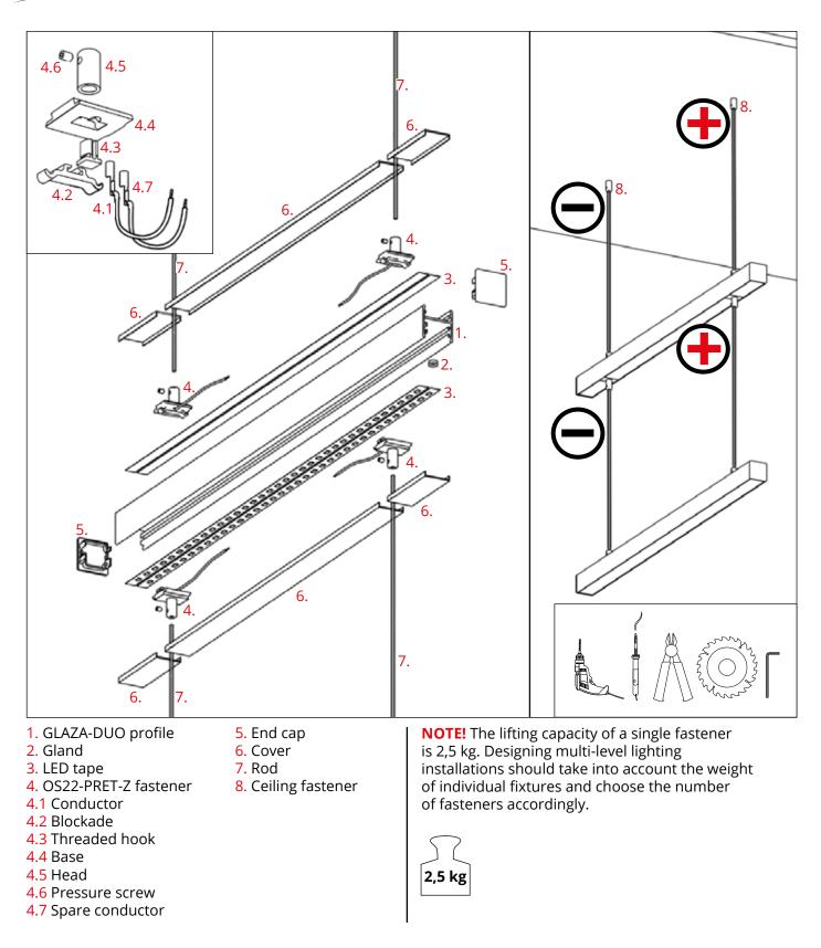
**NOTE!** All LED tapes must be connected to a 12 V or 24 V power supply.
