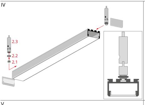
Fix the hooks (2.1) in the small channels of the profile, place o-rings (2.2) and wire sliding blocks (2.3) on them.
