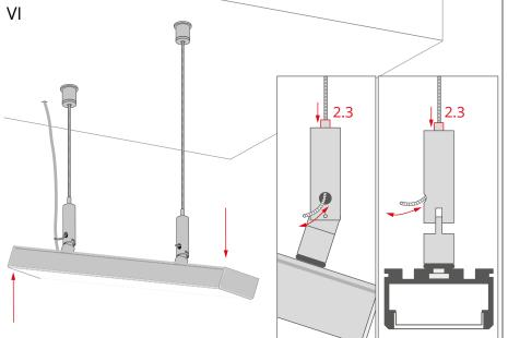
Suspend the lighting fixture and adjust the length of the wires with the blocks (2.3).
