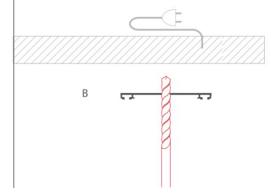
**3.** Attach the mounting track with screws (B). Insert clips (H) into it.
